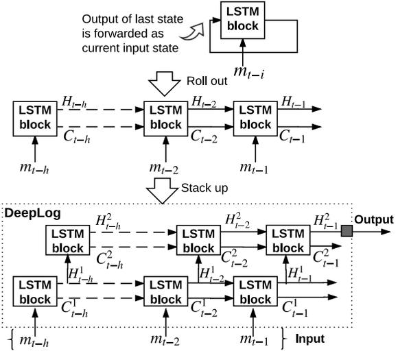
Figure 3: A detailed view of log key anomaly detection model using stacked LSTM.
